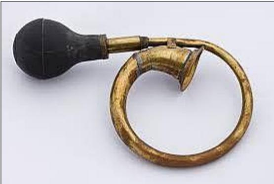
“The first type of hand-operated automobile horn was a kind of reed and bulb instrument, working somewhat on the principle of the organ. The vibration was produced by means of a nickel strip. The sound lacked penetration and had no continuous volume. This was before the days of the lead storage battery.
